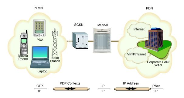
On traffic moving from the PDN to the PLMN, the MS950 inspects the IP packets to guarantee compliance with PDP parameter requirements. The packets are then mapped into GTP tunnels according to the destination IP address of the mobile subscriber (the PDP address) and forwarded to the corresponding SGSN. The MS950 administers subscriber state information that includes:
