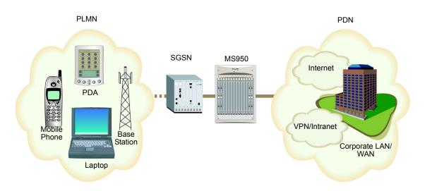
*Note:* The interworking functions between PDNs and PLMNs are assigned to the GGSN in General Packet Radio Services (GPRS) and Universal Mobile Telecommunications Service (UMTS).
